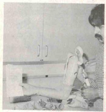
A small team of electronics technicians at the Fidelity the team's speciality, 'myonic' laboratories in specialises in designing and bionic, except that in a myonic building electronically con- arm the electrodes are mounted trolled arms and hands for over the muscles outside the amputees.
