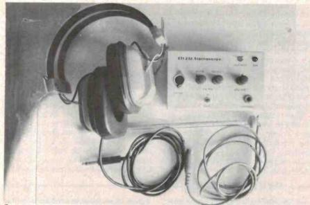
Completed stethoscope, ready for action! The probe here was made from a crystal earpiece, a length of 10 mm tubing being pushed over the ear plug.
