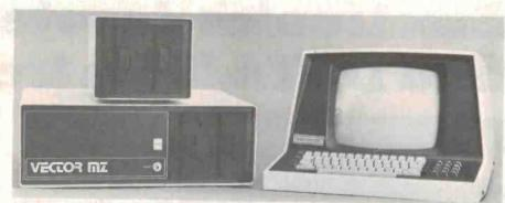
Sord systems are marketed in Australia by Mitsui Computer Systems. This is the M200 Mark VI, which features a 4 MHz Z80A CPU, 64K RAM and 8K ROM.
